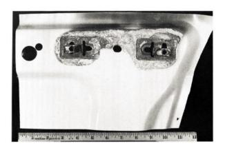
Galvanic corrosion of aluminum. A steel member (not shown in the picture) approximately the size and shape of the corroded region was in contact with the aluminum sheet.
