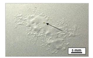
Filiform corrosion attack on aluminum part from a vehicle in service. The arrow points to the paint defect where the corrosion initiated.
