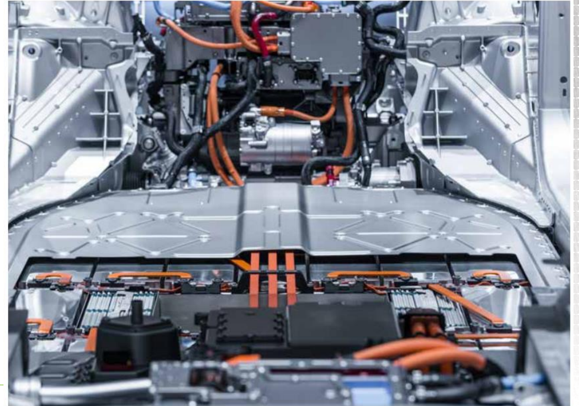
Battery tray in place in EV production line. (photo: Shutterstock)
